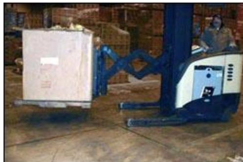
**Figure 11.** Reach trucks maximize maneuverability in narrow aisle.
