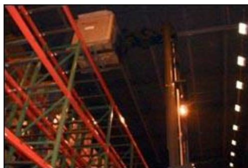
**Figure 12.** Triple reach extends 23 feet high. The lightest loads are placed on the top tiers.
