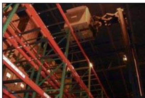
**Figure 13.** Reach mechanism extends forward to deposit load on top tier.
