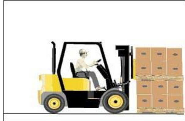
**Figure 8. Operator slides the forks into the pallet until they are fully under the load.**
