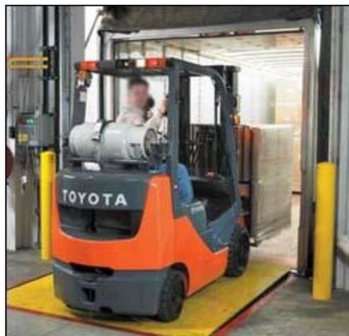
**Figure 16.** Operator using warning light and looking in the direction of travel when exiting a truck trailer.
