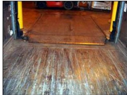
**Figure 18. Manual dock plate is secured into position. Always walk and inspect trailer floor before boarding.**
