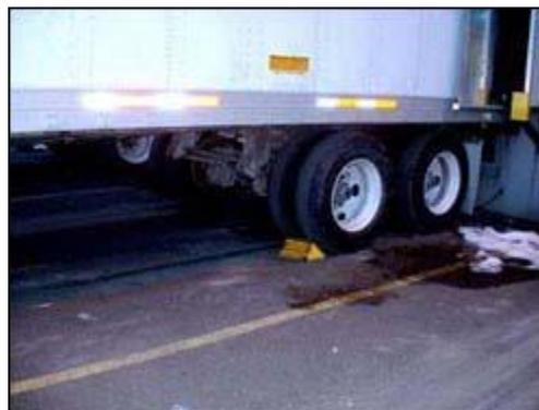
**Figure 14.** Wheels are chocked prior to boarding.
