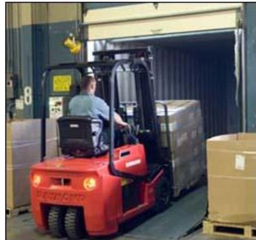
**Figure 17. Entering a truck trailer with adequate overhead clearance.**
