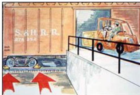
**Figure 15.** Use positive protection to prevent railroad cars from being moved.
