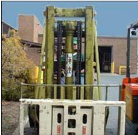
**Figure 3. Mast with central cylinder obscuring visibility.**
