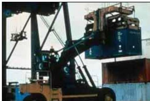
**Figure 5. Reach stacker used in marine terminals and longshoring.**
