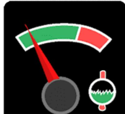
**Figure 5. Engine temperature gauge in the normal zone.**
