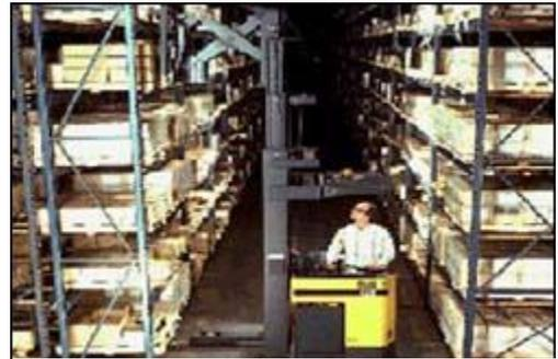
**Figure 2. Triplex mast in narrow aisle rider reach truck. Note that the forklift is removing stock from a rack. Foot and truck traffic in the opposite aisle way should be controlled to prevent injury from falling materials.**
