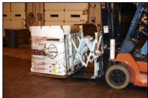
**Figure 2. Slipsheet attachment eliminates need for pallets.**
