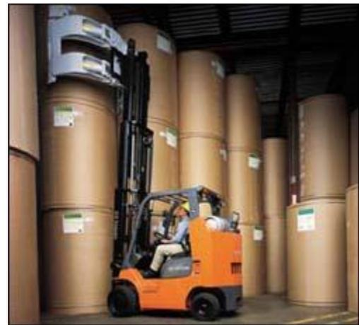
**Figure 4. Forklift equipped with a barrel clamp attachment.**
