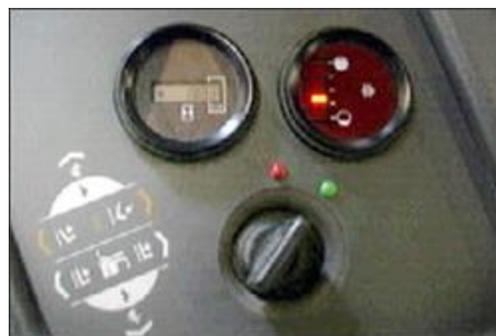
**Figure 2. These common forklift gauges show normal operating condition.**
