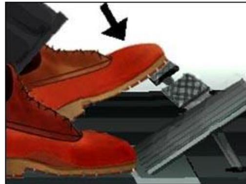
**Figure 1. Operator depressing inching pedal.**
