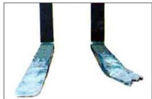
**Figure 2. Damaged fork.**
