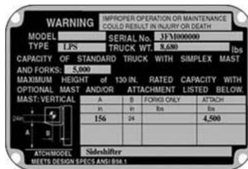
**Figure 1. This data label indicates that this forklift has a 156" upright mast height in column A and a 24" load center in column B. Its stated capacity is 5,000 lbs with just its forks. With the sideshifter attachment, its stated capacity is 4,500 pounds. The truck weighs 8,600 pounds.**
