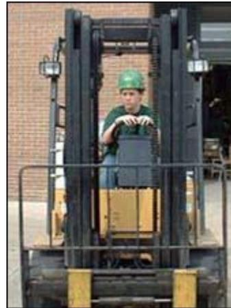
**Figure 4. High visibility mast with hydraulic cylinders on the sides.**
