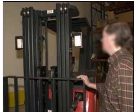
Figure 11. Operator performing operational inspection of working lights.
