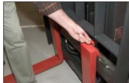
Figure 5. Operator inspecting the top clip retaining pin for the forks.
