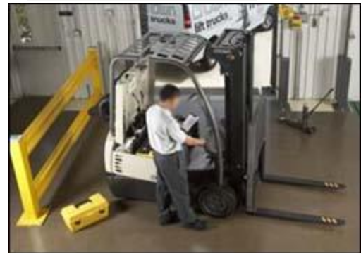
Figure 14. Preventive maintenance being performed on a forklift.
