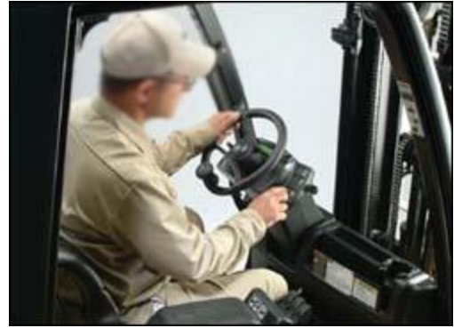
Figure 12. Operator conducting operational inspection with engine running.
