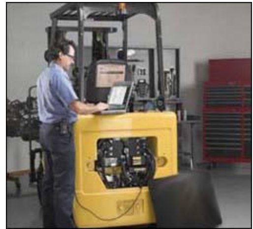
Figure 15. Technician conducting a diagnostic test of a forklift.
