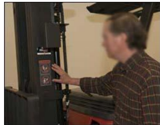
Figure 6. Operator ensuring that warning decals are in place and legible.
