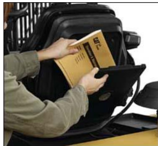
Figure 9. Operator ensuring that the operator manual is on board the forklift and legible.
