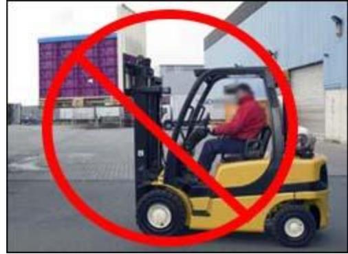
**Figure 15. Do not travel with the load elevated.**
