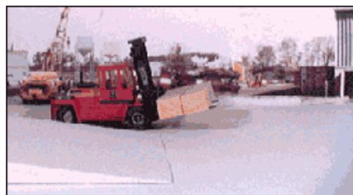
**Figure 7. Forklifts are less stable on turns and grades and can tipover.**
