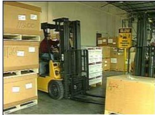
**Figure 5. Operator slows down and sounds the horn at cross aisles where vision is obstructed.**
