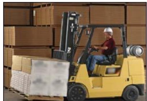
**Figure 14. Operator traveling with load lowered.**
