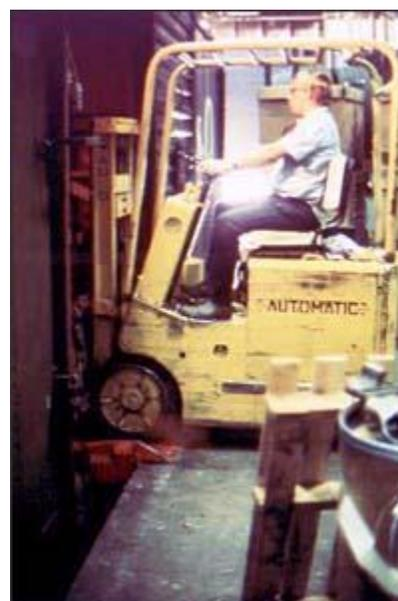
**Figure 2. Use curbed ramps and dockboards to keep lift trucks from sliding.**
