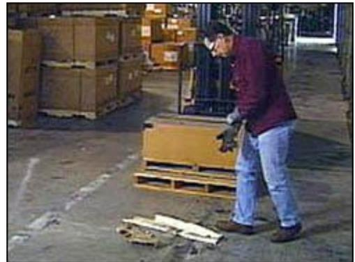
**Figure 4. Get off the forklift and remove the obstruction.**
