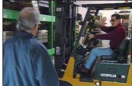
**Figure 7. Operator signaling to coworker to stand back.**
