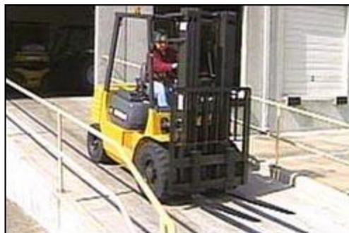
**Figure 7. Traveling down ramp without load.**
