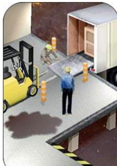
**Figure 1. Do not drive over oil and grease spots. Use a dock board or plate to bridge the gap between the dock and the truck being loaded or unloaded.**
