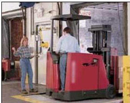
**Figure 3. Paint the edges of loading docks to improve visibility. Check for pedestrians, over vehicles, and other obstacles when exiting trailers.**
