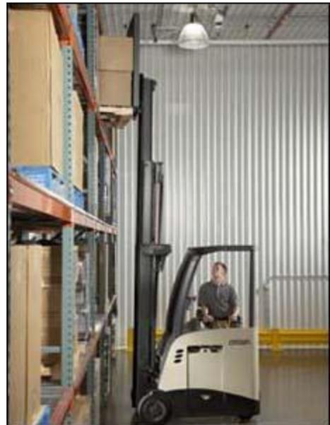
**Figure 6. Ensure adequate overhead clearance.**
