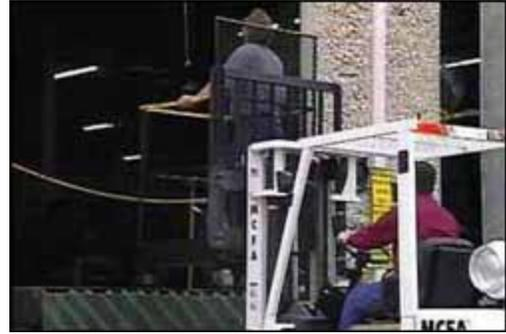
**Figure 6. Specialized platform for lifting coworker. Note: There is a guard on the back of the platform to keep the person in the platform and protect the worker's arms and hands.**
