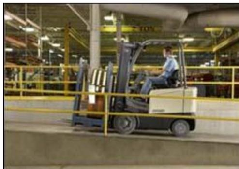
**Figure 1. Drive loaded trucks forward going up a ramp.**
