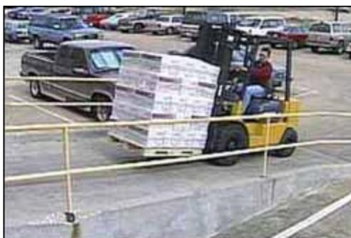
**Figure 4. Traveling up ramp with load.**
