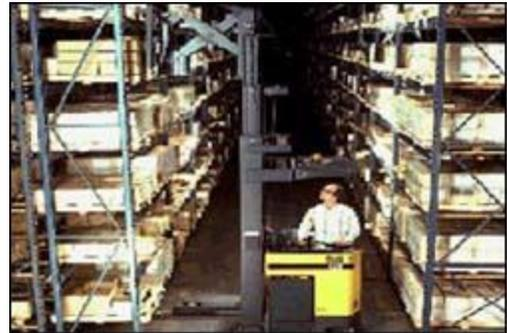
**Figure 2. Reach truck with pantograph attachment that scissors forward from the mast to retrieve the pallet.**
