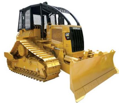
At the end of the shift, clean the tracks properly. Clean any build-up around the track rollers, track slides, and the tracks; removing mud, snow, slush and ice will prevent the material from freezing overnight. Also, grease the machine while the components are still warm; joints will take grease better because they've been moving. (The grease gun can be kept in the operator's cab while working to keep the grease warm.)
